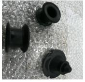
11. Lubricate rubber bushings and install on new air box.
