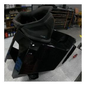
14. Install supplied rubber edge guard on half round section of new airbox and trim accordingly. Mock up before trimming to ensure the correct length is cut.
