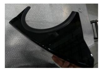
30. Install lid on airbox using supplied hardware.
