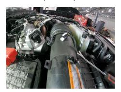
3. Lift coolant hose out of clip connection.
