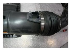
19. Install MAF sensor in new intake tube and make sure it is facing right direction before tightening down with supplied hardware. **NOTE**: The arrow on the MAF sensor needs to point the same direction as the air flow through the intake or it will throw a CEL.
