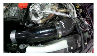
26. Install air filter into air box with open end facing up and lift up slightly on intake pipe while positioning air filter in place.
