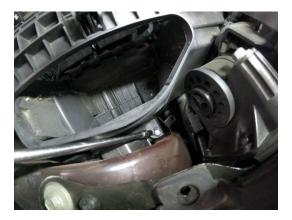
9. Lift and remove air box up out of engine bay.
