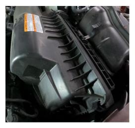
6. Remove intake tube with air box lid and then remove air filter.
