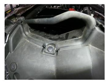
18. Remove MAF sensor from original intake tube.
