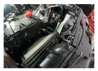
7. Remove pushpin holding the air box snorkel in place and remove snorkel.
