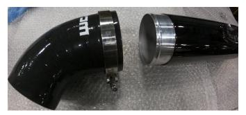
22. Install boot and clamp on new intake pipe and make sure airflow direction of MAF sensor is correct. **NOTE**: When installing the boot, the arrow on the MAF sensor needs to point the same direction as the air flow through the intake or it will throw a CEL.
