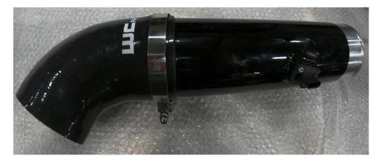
23. Using both hands, shape provided hose clamp into place around oval side of boot.
