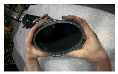
24. Install air filter outerwear cover on new filter.
