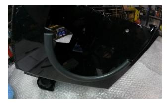
15. Set airbox in place & ensure front lower air duct lines up with airbox when air box is slid into place.
