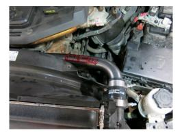
9. After everything is in place and tightened down, a pressure test of the cooling system is recommended. If you don't have access to one, you can get the truck up to temperature and inspect for leaks. After a few drive cycles, it is best to recheck t-bolt clamps to ensure they are still tight and no leaks are present.
