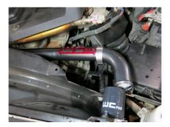
7. Using screwdriver or pick, run boot around the end of the pipe while pushing into the boot.
