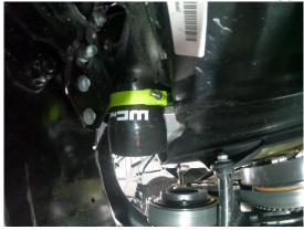
8. Install boot onto turbo but don't tighten clamps yet.
