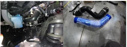
16. Clean both intercooler connection points at intake air valve and intercooler. Install new boot at intercooler outlet and tighten clamp at intercooler connection only.
