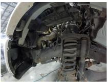
15. Remove clamp at driver side intercooler connection working through inner fender area. Remove pipe from truck.
