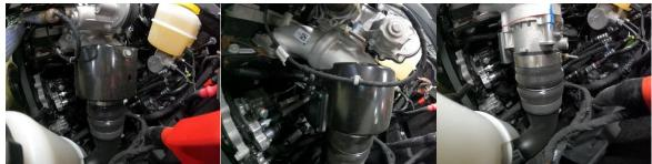
13. Remove intercooler boot clamp at intake air valve.
