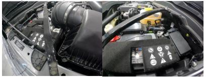
3. Remove air box lid, tube, and lower air box.
