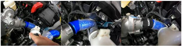
18. Tighten all clamps for driver side pipe at top and bottom connections.
