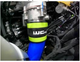
19. Boost testing the system to verify all new connections are leak free as well as the rest of the system is strongly recommended to ensure maximum performance and functionality. We also offer a boost tester on our website (Part# 13U7H001).
