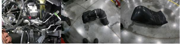
4. Loosen intercooler pipe clamp at turbo outlet.
