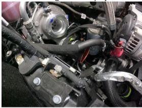
9. Install pipe as shown with intercooler side lined up and start pipe into boot on intercooler connection. Then, pull boot at turbo side onto the intercooler pipe using a hook tool for assistance, just be careful not to damage boot.
