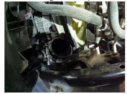
17. Use Dr. Tranny's Assemblee GOO or similar product on both ends of intercooler pipe to aid install of pipe into boot on intercooler. Make sure clamps are on pipe so they can be slid up to the boot once it is in place. Longer end of pipe will go to the intercooler.
