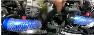
10. Center the pipe and boots to allow for correct clamp installation. Make sure the clamp sits past the beadroll to avoid blowing off while driving. Tighten all the remaining clamps that have not been previously tightened.
