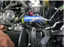
11. Reconnect grid heater and alternator wiring connections and reinstall intake.
