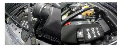
3. Remove factory airbox & tube from truck. There will be one clamp at turbo inlet and one clamp at airbox. Next, remove the air duct from cowl before removing lower box. Once these are all taken off, pull straight up on the box to remove it.
