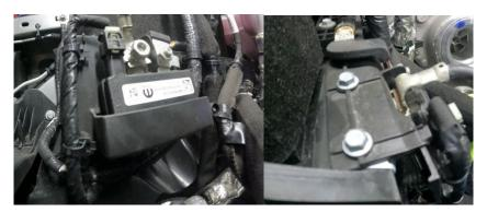
7. Remove air box lid and install rubber insulator onto box & lid, then trim as shown in pics below to desired length.
