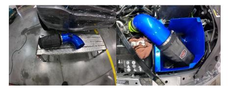
10. Reconnect sensors on intake pipe and install airbox lid with 4 supplied button head screws.
