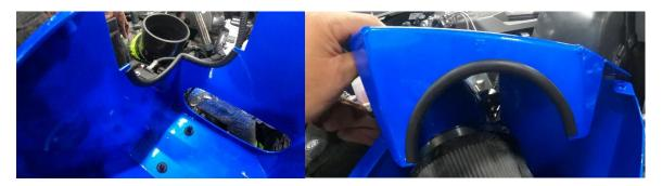
8. Transfer air duct and rubber isolators from old box to new box (top right picture) and Install into place on side bracket and bottom of box. Check clearance with high-pressure ac line and transmission lines on the front corner of the box near fender. Once fitment is verified, install the ram air duct (shown out of truck for visual).
