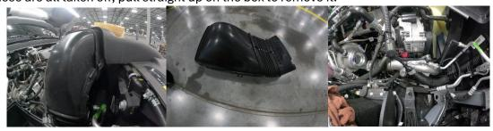
4. Install supplied boot on turbo and tighten clamp at turbo inlet.
