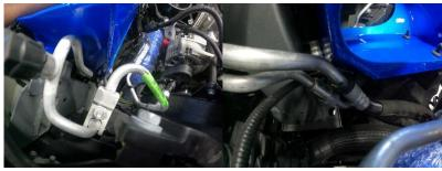
9. Install air filter onto tube & slide tube into boot at turbo inlet & tighten clamps. Clamp should be just past the bead roll and tightened by hand until boot indents. Make sure filter is also seated just past end of pipe and no further. If filter is pushed too far on to pipe, it will limit air flow.
