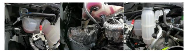
9. Remove the coolant tank nuts (three 10 mm nuts).
