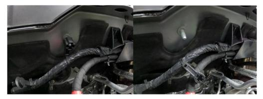
13. Use a hook tool to remove top lines from OEM coolant tank and transfer to new WCFab tank utilizing the new provided hose clamps. Transfer AC line bracket to AC line & reconnect with 10mm bolt. Reconnect level sensor at this point as well.
