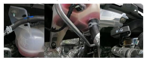
10. Remove the coolant tank from engine bay.
