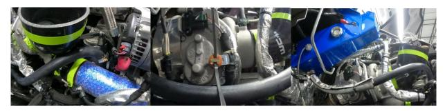
16. Install the overflow hose on nipple at fill neck and route it down into fender area.
