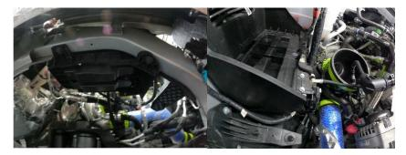
7. Remove the coolant tank top lines and save for install of new WCFab tank.
