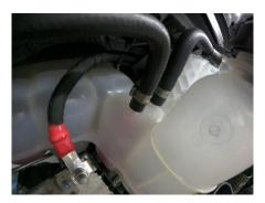
8. Remove coolant tank lower hose and disconnect level sensor plug. There will be one 10mm bolt for AC line bracket.
