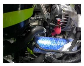
15. Install new hose & trim to correct length. Use zip tie to hold hose & heat wrap in place.
