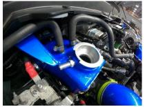
14. Remove OEM hose from engine side as shown below.
