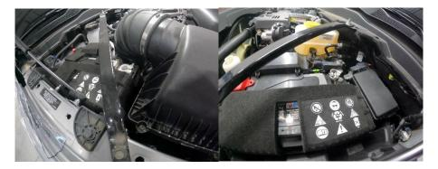
2. Drain coolant. This is at driver's side of radiator near bottom. You can then reach down to it from top of engine bay. Remove coolant tank cap for fast drain.
