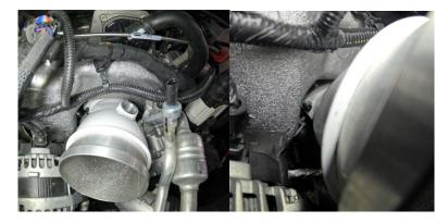
11. Reconnect PCV line to supplied threaded bung on your new intake horn & reconnect AC sensor.
