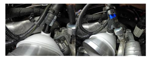
12. Reinstall airbox and intake tube.
