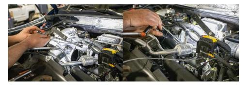
6. Remove factory intake horn.
