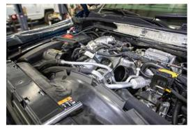
3. Remove valve cover breather hose from intake horn by twisting and pulling up at the same time. Usually, the metal clamp can stay in place and you can slide directly on to the new intake horn.
