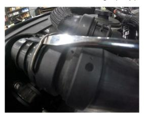
3. Remove radiator hose after clips are removed.
