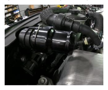
7. Slide one clamp onto each side of coolant pipe as well as onto each adapter on truck.
