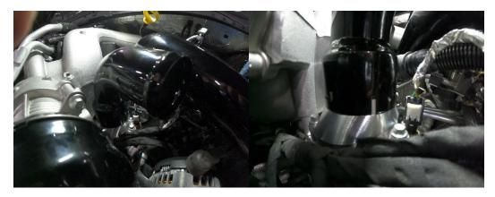
6. Install straight adapter on radiator side, making sure notch on side lines up as well. Make sure adapter is fully seated onto radiator & clip is seated in place.
