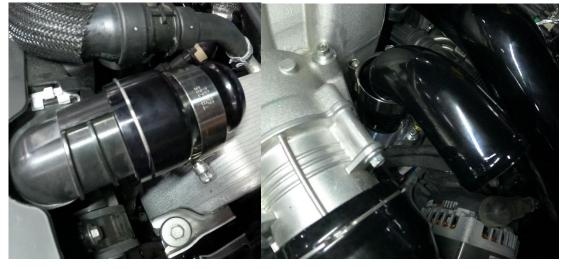
8. Install boots on each end of coolant pipe (lube on boots eases install) and clamp in place.
