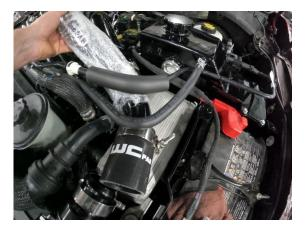
10. Install at thermostat housing, followed by radiator side and tighten existing clamps in place.
