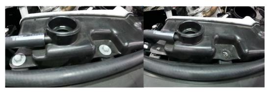
5. Lift tank up and away from radiator to access small coolant hose.
