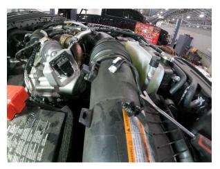
12. Reconnect the batteries and start the engine and run at idle for about 15 minutes to check for leaks and let air escape from the cooling system.
