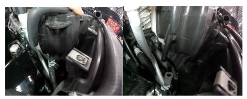
6. Remove original tank from engine bay.
