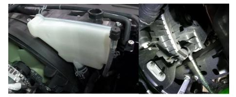
3. Remove clamp and upper coolant hose.
