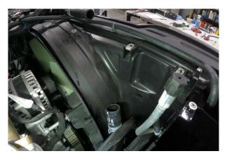
7. Set new tank in place of original and reinstall larger hose first, followed by smaller hose. Make sure lower tab fits into pocket on fan shroud and mount in place with supplied hardware (Qty 2: M6-1 X 16mm Screws).
