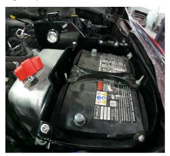
30. Remove plastic shield from battery cables.
