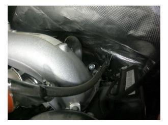
7. Disconnect sensor from hot side charge pipe (HO Models) and remove charge pipe starting at turbo side.
