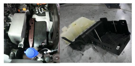
16. Install new supplied M8 J nut onto battery box tab for intercooler.
