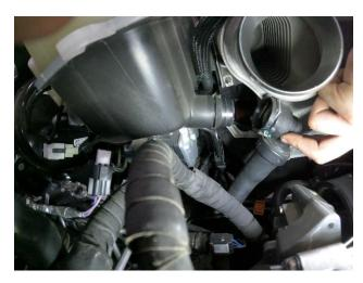
12. Remove two 13mm mounting bolts from battery box to intercooler.
