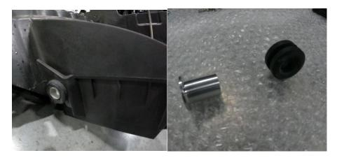
18. Install rubber busing into new battery box, then install supplied sleeve into rubber busing from the inside of battery box.
