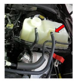
9. Unclip vacuum line connector and remove clip from coolant tank. Then you can unclip vacuum solenoids from rear of tank and push back.
