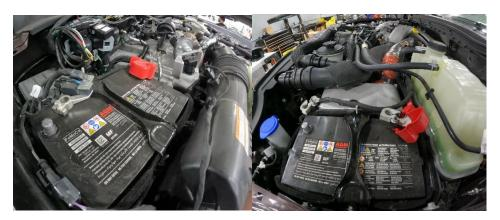
2. Remove battery hold down bracket and remove battery.
