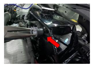
33. Reconnect vacuum line to port behind coolant tank.
