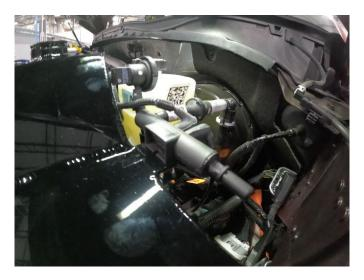
26. Wrap supplied larger isolator clamp around vacuum solenoid with tab facing engine.
