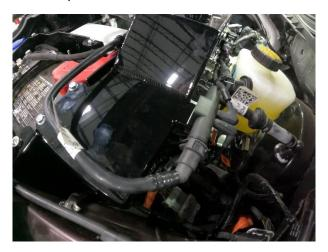
34. Install coolant overflow hose, some trimming may be required for perfect fitment.
