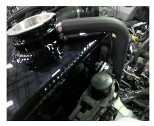
35. Reinstall hot side charge pipe.
