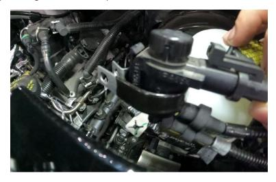
27. Use shorter M6x12mm bolt to mount vacuum solenoid to back of coolant tank.
