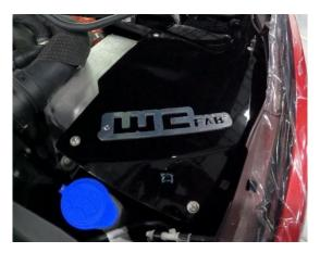
39. Top off the cooling system and start the engine. Run at idle for about 15 minutes to check for leaks and let air escape from the cooling system. Install the cap and test drive. Please note you have to top off the cooling system a few times, as air may still be in the system.
