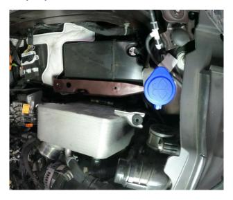
14. Remove four 13mm mounting bolts from battery box.
