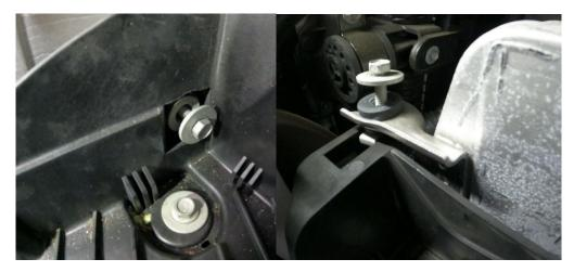
13. Lift intercooler up until lower tab clears its pocket, then push intercooler towards engine and away from battery tray.
