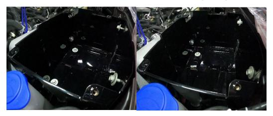
$20.\ Lift\ intercooler\ back\ into\ position,\ making\ sure\ lower\ alignment\ tab\ is\ fully\ seated.$
