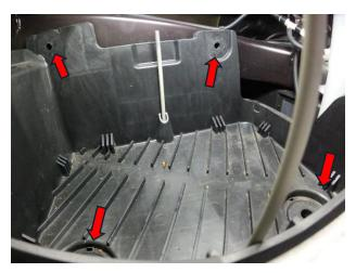
15. Lift battery box/coolant tank assembly up and out of truck.
