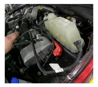
10. Unclip battery cable retainer from coolant tank and set cables to the side.
