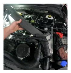
5. Release the locking clip at the hot side charge pipe turbo connection using two long flat blade screwdrivers.
