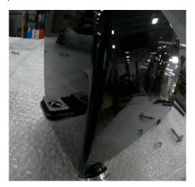
23. Set coolant tank into position & use supplied M6 hardware to mount coolant tank, but don't fully tighten them yet.
