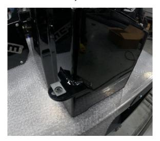
17. Remove rubber bushing from intercooler mount on original battery box.
