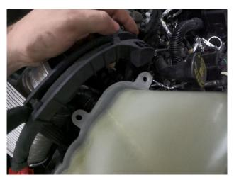
11. Disconnect lower coolant hose from tank.
