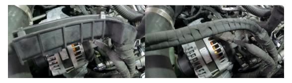
31. Install small isolator clamp on battery cables & secure to tank with supplied M6 bolt.
