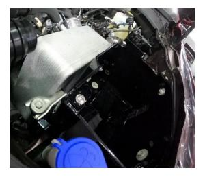
21. Secure intercooler to battery box with one OEM bolt and supplied 13mm M8 bolt through rubber bushing.
