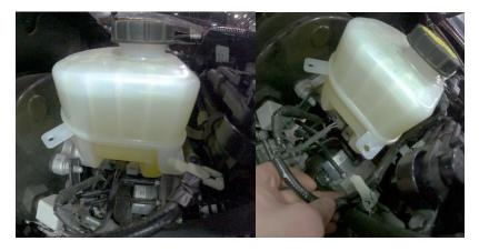
2. Install both included clip nuts on plastic tabs on driver side of brake reservoir.
