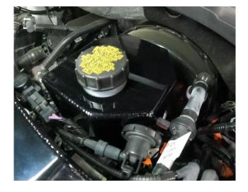
6. Install supplied hardware (Qty 2: M6-1 X 16mm Screws) and tighten in place.
