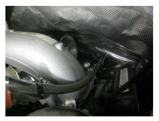
5. Disconnect sensor from charge pipe if equipped (only on High Output Models) & remove pipe starting at turbo side.
