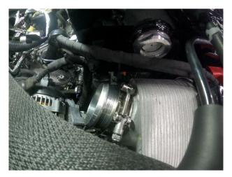
11. Install new charge pipe at turbo connection and push until wire retaining clip locks in place.
