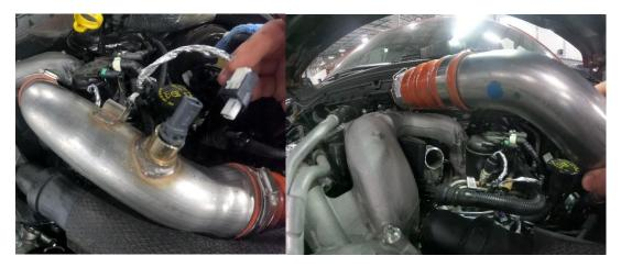
6. Transfer sensor to new charge pipe.
