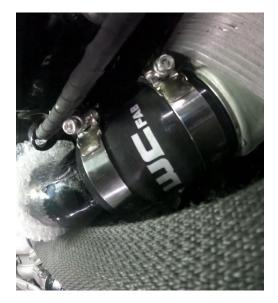
14. Connect sensor and tuck any extra wire out of the way Then set dipstick in place and reinstall 10mm bolt and nut.
