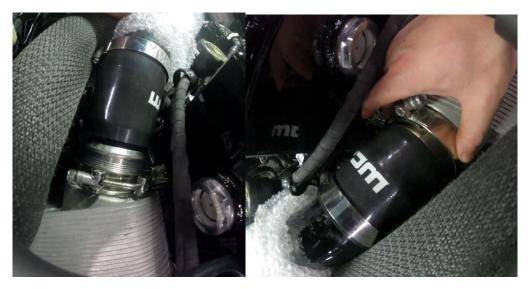
13. Adjust both clamps & boot with equal boot gap on pipe and intercooler side and tighten them in place. At this pont, a microfiber towel and degreaser can be used to clean excess assemble goo from install.
