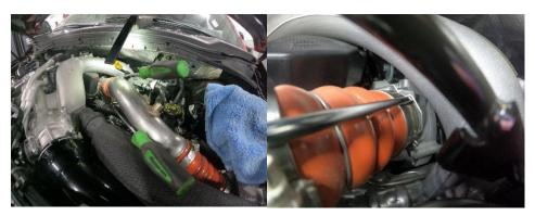
4. Remove the 10mm bolt and 10mm nut holding dipstick in place and move it aside. Dipstick can be fully removed to allow more clearance as well.
