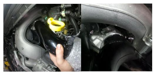
12. With charge pipe in place, slide boot off pipe and onto intercooler connection, aligning clamps at the same time.
