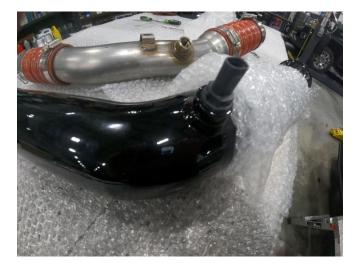
7. Install provided o-rings into charge pipe dry & make sure they're fully seated before applying some lube onto installed o-rings (Dr Tranny's Assemble Goo works well).
