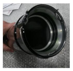
9. Slide one clamp onto pipe followed by supplied boot (slide boot all the way onto pipe) with some lube to ease install. IMPORTANT: Boot can be damaged if Dr Tranny's Assemblee Goo isn't used.
