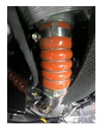
3. Release the locking clip at the turbo connection using two long flat blade screwdrivers.
