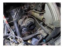
4. Remove sensors from original intake tube and install them into new intake pipe.
