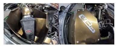
10. Tighten intake tube clamp on turbo side, then slide ccv hose onto pipe coming from the engine and tighten clamp.
