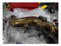
5. Install CCV hose onto new intake pipe and tighten clamp.
