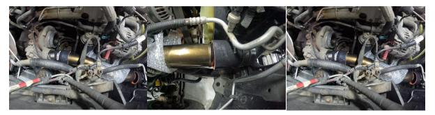
8. Tighten the remaining clamps when proper positioning has been achieved.
