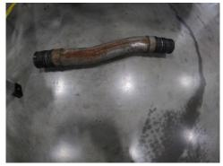
6. Clean turbo outlet to make sure it is free of any oil or debris, install new boot on turbo outlet and only tighten clamp at the turbo. Use Dr Tranny's Assemblee Goo or similar product to help slide the new boot on the intercooler inlet past the stops for the original boot.
