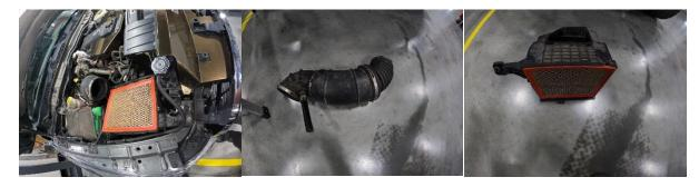
5. Loosen the passenger side intercooler clamps at the intercooler and turbo outlet, remove the pipe from the truck.
