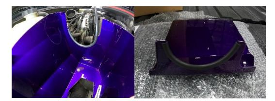
21. Install outerwear cover on air filter, then install filter on intake pipe 2" in from beadroll and tighten clamp
