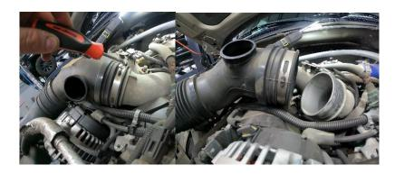
6. Remove MAP connector and alternator wiring for better access to intake horn bolts.
