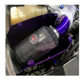
22. Reinstall MAF sensor into new intake pipe (arrow on bung points in airflow direction to turbo) and reconnect wire harness to it.
