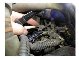
14. Install intake horn on two lower bolts installed previously.
