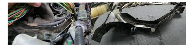
12. Tape harness to assist with install of wire loom.
