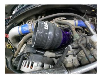
19. Install lower airbox using hardware from OEM airbox
