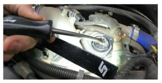
8. Install two lower bolts from supplied hardware.
