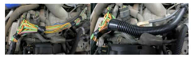
13. Cut tape on alternator harness to MAP sensor.
