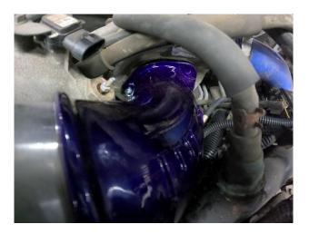
15. Thread in the third bolt and tighten them all down to secure horn to turbo face.
