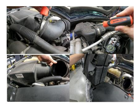
4. Remove the resonator box from the top of the engine by removing screw at back connection and clamp to intake.
