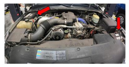
2. Disconnect MAF sensor from OEM intake.
