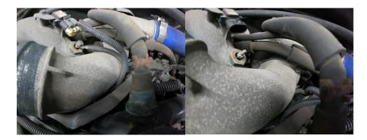
7. Remove all three 10mm bolts from intake horn and carefully clean gasket from turbo face.
