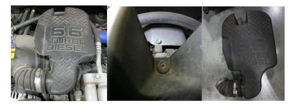
5. Remove intake pipe from intake horn by loosening clamp connection.
