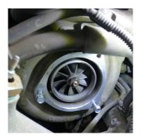
9. Some Dr Tranny's Assemblee Goo (example below) can be used to hold o-ring in place on intake horn. Assemblee Goo can be found online or at local auto parts store.
