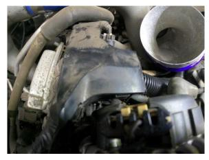
17. If wire track is broken, tape and install loom in shown location.
