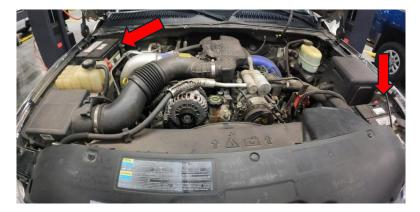
2. Disconnect MAF sensor from OEM intake.
