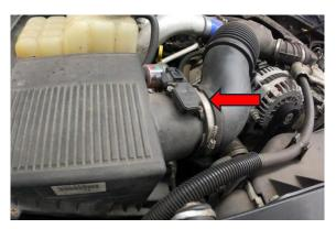
3. Remove factory upper and lower airbox from engine bay. A flathead screw driver can be used to remove clamps and then pull up and remove in one piece once clamps are off.
