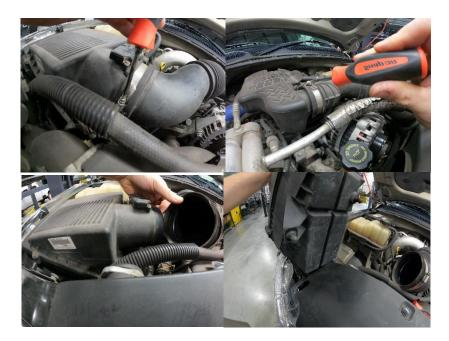
4. Remove the resonator box from the top of the engine by removing screw at back connection and clamp to intake.
