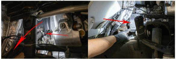
6. Remove the EGR valve and temperature sensor from the manifold. Push both up and tie up and out of the way.
