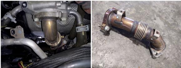
Remove bolts from the passenger valve cover heat shield and the foam insulator to allow for access to the up pipe bolts at rear of exhaust manifold.
