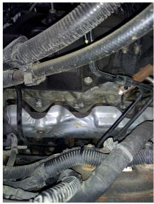
23. Remove the manifold heat shields.
