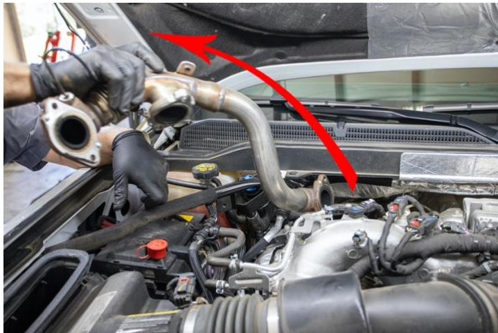
17. Remove EGR Pipe and set aside being careful not to damage riveted on gaskets which will be needed for reinstallation later.
