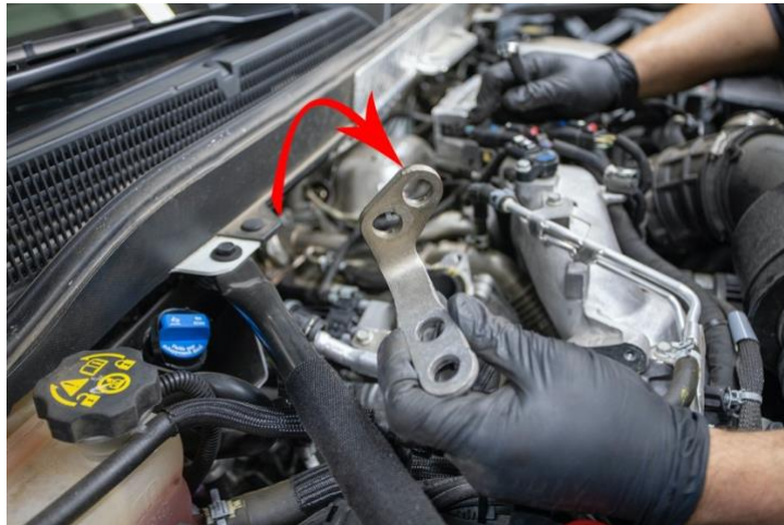
28. Reinstall upper downpipe bracket.
