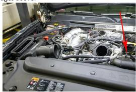
4. Remove resonator and intake piping and set aside for later re-installation.
