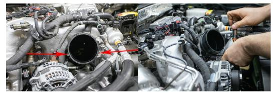
5. To remove OEM intake horn, locate and remove bolts shown in images above. This can be done using a long ¼" extension and 13mm swivel socket. There is no reason to remove any other items for access.
