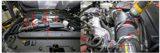
3. Disconnect intake pipe and resonator assembly by disconnecting clamps and fasteners at the points indicated in the images above.
