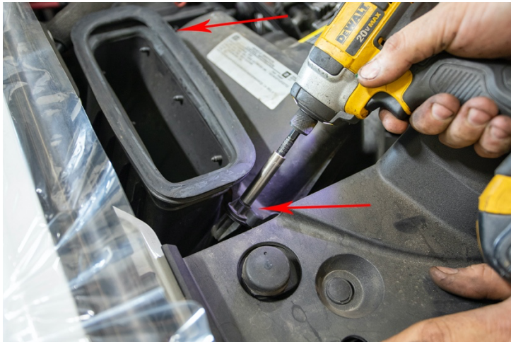
5. Unplug MAF Sensor and disconnect intake pipe
