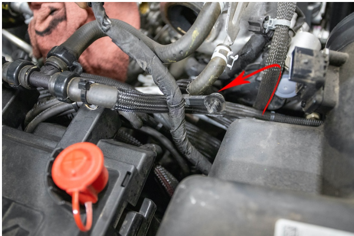
7. Remove Wire Harness Clip and tuck safely out of the way.
