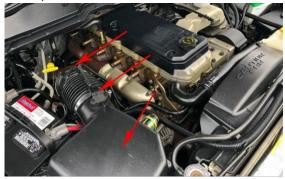
5. Remove OEM air Intake. Remove MAF sensor and save for later reinstallation.
