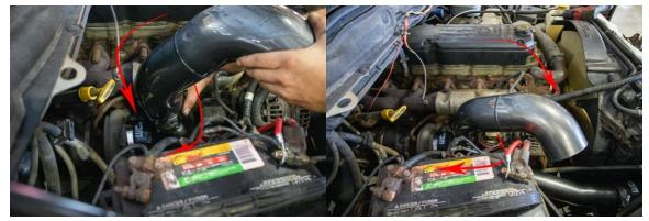
10. Install lower intake pipe end into turbocharger inlet boot and clamps first.
