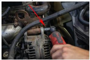
7. Using a 15mm socket loosen the upper alternator bolt to make space for the intake support bracket. Do not remove.
