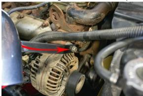
11. Adjust pipe as necessary to slide intake support bracket onto alternator bolt and adjust pipe to turbo boot connection to ensure proper sealing and clamp placements to the pipe bead roll. Retighten alternator bolt.
