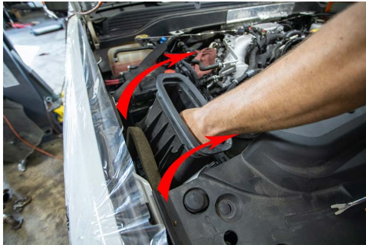
25. Separate Lid from Airbox. Grab Lower Airbox and pull up firmly to unseat the lower airbox from the inner fender.
