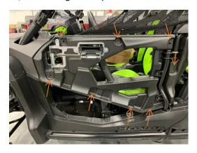
2. Drill four ¼" horizontal holes into the pre-existing factory markings.
