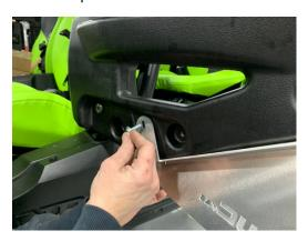
5. Insert 7/8" bolts in the remaining 3 holes. Make sure all washers, nuts and bolts are in and tighten.
