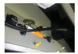
9. Remove the light (two T-20 screws).
