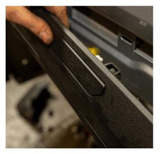
11. Reinstall the clips to the fender.
