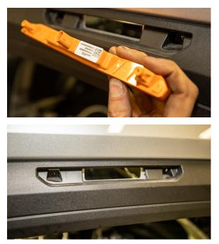
Install the WC Fab delete into the truck and used supplied hardware (not the factory T-20).
