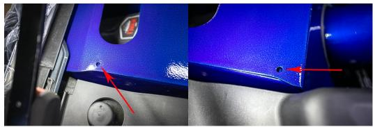
26. NOTE: When installing upper lid of your intake air box some amount of misalignment may occur between the box and lid as shown in the images above. Follow steps below to properly adjust alignment and complete your installation. Do not force screws into holes.
