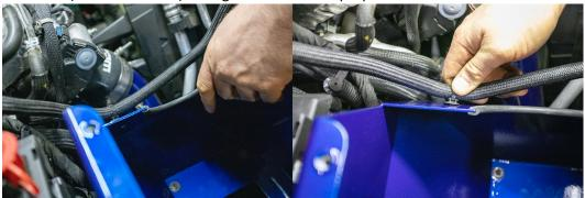
Install supplied pipe seal on lower air box and trim to fit saving excess for use on the lid in Step
