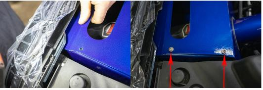
27. Adjust lid to align front air box mounting holes and loosely install supplied fasteners to locate the assembly.
