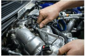
22. Reinstall coolant hardline.
