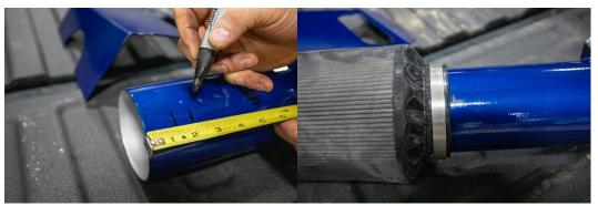
17. Using a tape measure and a marker, place small mark at 2" from filter end of your new intake pipe to help set mounting depth. Install filter onto pipe leaving mark exposed. **Improper filter depth can cause air restriction on your new intake.** Do not tighten filter clamp at this time.
