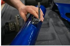
18. Remove MAF sensor from OEM air intake and reinstall on your new air intake pipe using supplied hardware and maintaining correct orientation. The OEM MAF sensor screws will not work. Do not try to install them on your new pipe.
