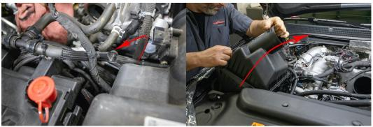
6. Remove coolant line clip and tuck safely out of the way. Next, remove OEM air box. Grab and pull up firmly to unseat from the inner fender.
