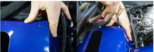
28. With front fasteners in place, adjust lid and air box wall to align holes and install rear fasteners.
