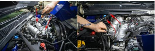
8. Unbolt retaining tabs (2x 10mm bolts) shown. Shift coolant hardline gently out of the way to provide clearance for new air box installation preventing scratches to the powder coat finish.
