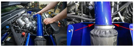
23. Install Intake pipe with filter assembly into hump boot at horn and adjust pipe placement and filter depth as necessary to allow a gap as shown in image above between filter and air box seal.
