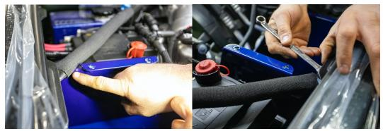
13. Note: Build tolerances vary from truck to truck. Many trucks will require no adjustments for your air box installation. However, on some trucks, the fender brace may contact the air box as shown in this image. To correct this, first loosen the brace at the fender using a 13mm wrench.
