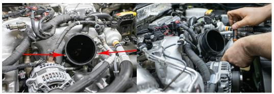
19. To remove OEM intake horn, locate and remove bolts shown in images above. This can be done using a long ¼" extension and 13mm swivel socket. There is no reason to remove any other items for access.
