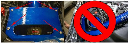
29. Tighten air box lid fasteners in a clockwise pattern starting at the front left fastener and finishing at the rear left fastener. Locate the supplied ram air hood seal. THIS SEAL IS FOR THE BOTTOM OF YOUR HOOD RAM AIR DUCT. IT DOES NOT GET INSTALLED ONTO YOUR AIR BOX LID.
