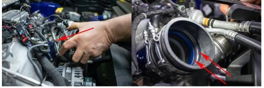
21. Install hump boot and clamps onto intake horn paying close attention to match alignment of horn lip to hump shown as indicated in image above.
