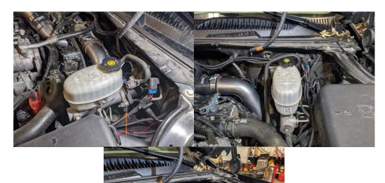
Loosen the two 15 mm nuts on the front of the master cylinder. If the stud starts to rotate, hold it on the back side with a wrench while loosening and tightening the nut.
