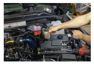
3. Remove the lower clip style hose from the coolant tank.
