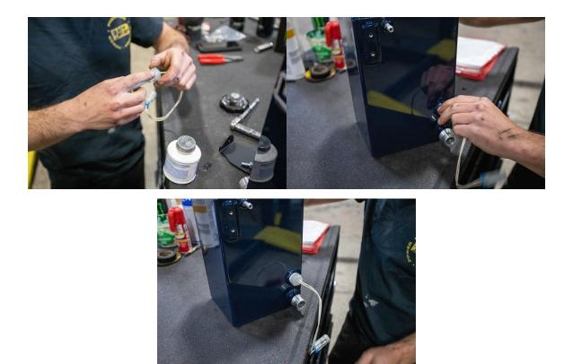
12. When properly installed, the sensor should not have threads showing, just like the picture shown. The arrow on the sensor faces up to make sure the sensor will function. These are pipe threads and need to be tightened all the way to seal up.
