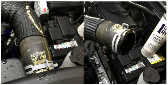
5. Repeat this process at the thermostat housing and remove the hose from the truck.
