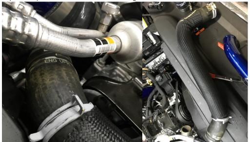
6. Install the boots and loosely install the clamps at both the radiator and the thermostat housing.
