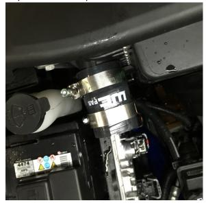
7. Install the pipe into the boots at both ends. You can now align the boots and clamps for proper logo placement and clamp orientation. (Be sure to allow proper clearance for tightening)
