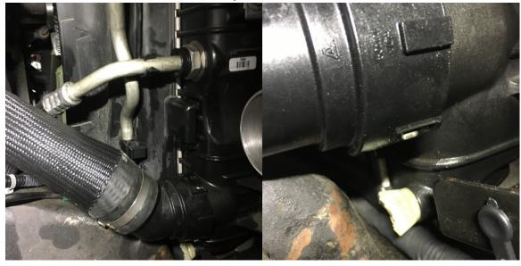
4. Release the tension on the clamp for the upper radiator hose at the radiator and remove the hose from the radiator.
