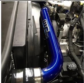
9. Check for leaks before driving and tighten t-bolt clamps if needed.
