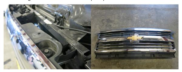
4. Remove front bumper. There are four bolts in the center and one on each end in front of the tires. Disconnect the wiring harness underneath the bumper towards the passenger side. The Bumper harness stays on the bumper for removal. Unplug fog lights if equipped. Lay bumper face down on cardboard or towel.
