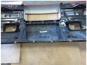
5. Remove lower valance metal support. There are six upper 15mm bolts and six lower 10 mm bolts.
