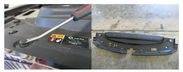
3. Remove grille. There are four bolts on top and push disconnects.
