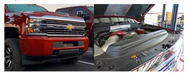
2. Remove plastic radiator cover under hood by removing twelve plastic pop rivets to reveal radiator stack.
