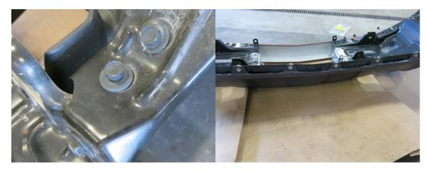
6. Remove both bumper support brackets and fog lights from each side of the bumper. There are five 15 mm bolts on each side.
